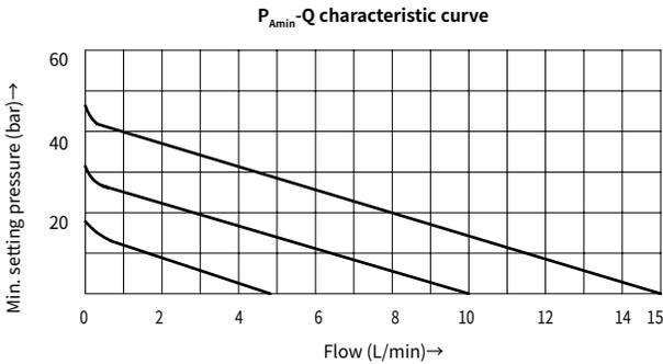
**$P_{Amin}$ -Q Characteristic curve shows the flow-rate in relation to the adjustable min. pressure rating from P to A.**
